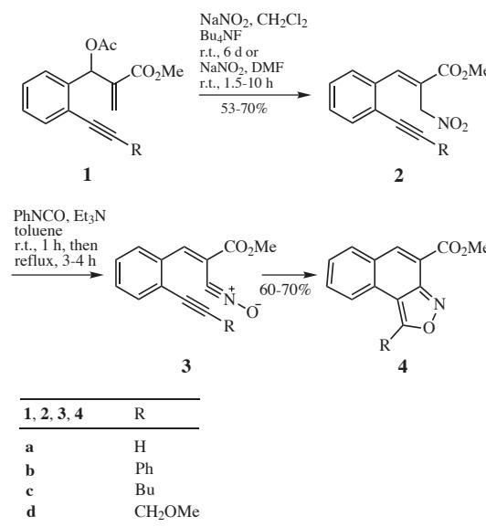
The readily available *o*-acetylenic Baylis-Hillman adduct acetates **1a-d**, whose preparation has been previously described [23], provided a convenient starting point for the synthesis of this ring system, as shown in Scheme I. Treatment of Baylis-Hillman acetates **1a-d** with sodium nitrite in *N,N*-dimethylformamide at room temperature for 1.5-10 hours afforded *o*-acetylenic 2-nitromethylcinnamic acid methyl esters **2a-d** in 20-70% yields [17b]. A better
